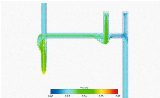
Figure 8. The flow pattern with velocity vectors in the STM. The velocity is indicated by the length and colour of the vector. It clearly shows that the simulation gives the desired flow as set-up with the model and that the ratio of mixing is 1:1 in the right side of the STM. The units are arbitrary.
